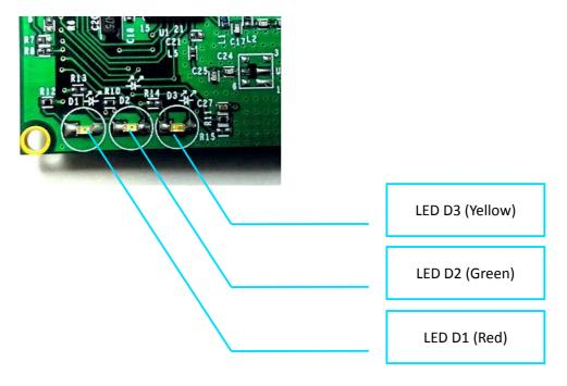
The pin details of the LEDs are as follows:
